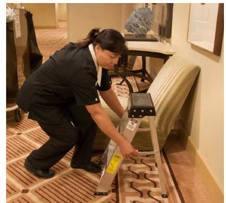
Before climbing a step ladder, position all 4 feet on a firm, level surface and lock the spreaders.
